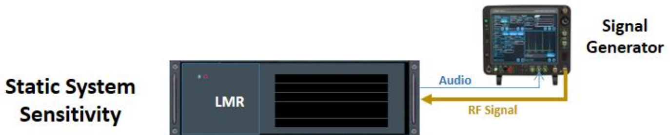
Figure 5: Static Sensitivity Testing of a receiver
