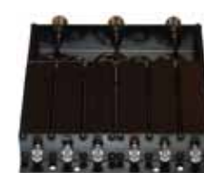
DSD706M 6 Cavity Multi-Channel Mobile Duplexer
