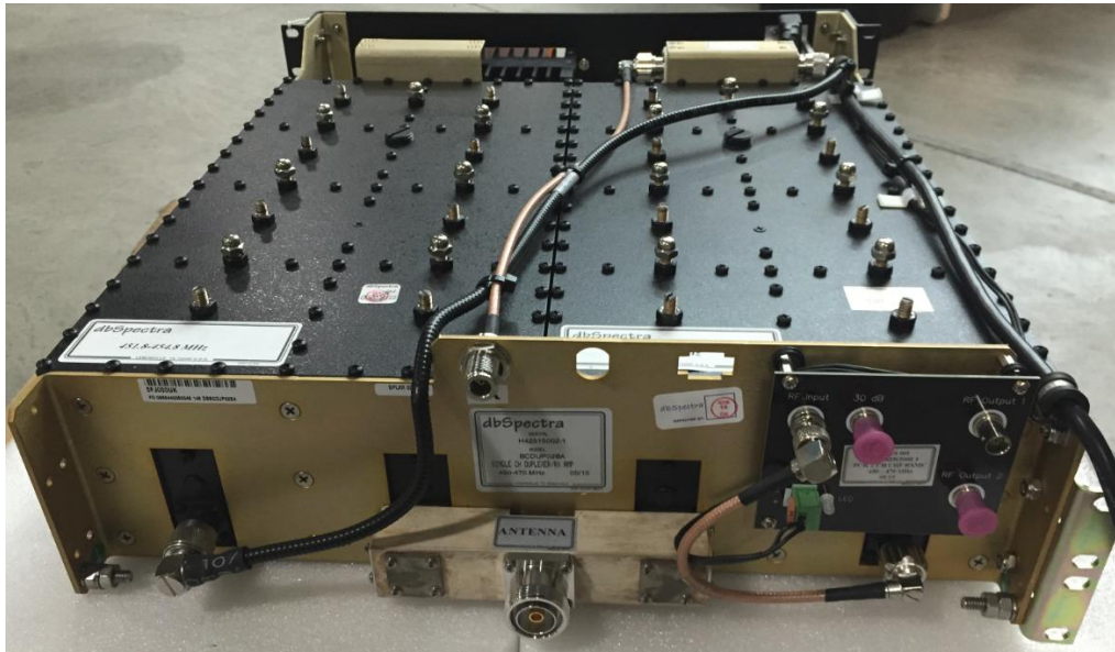
Figure 17: Example of a single Channel Duplex System
