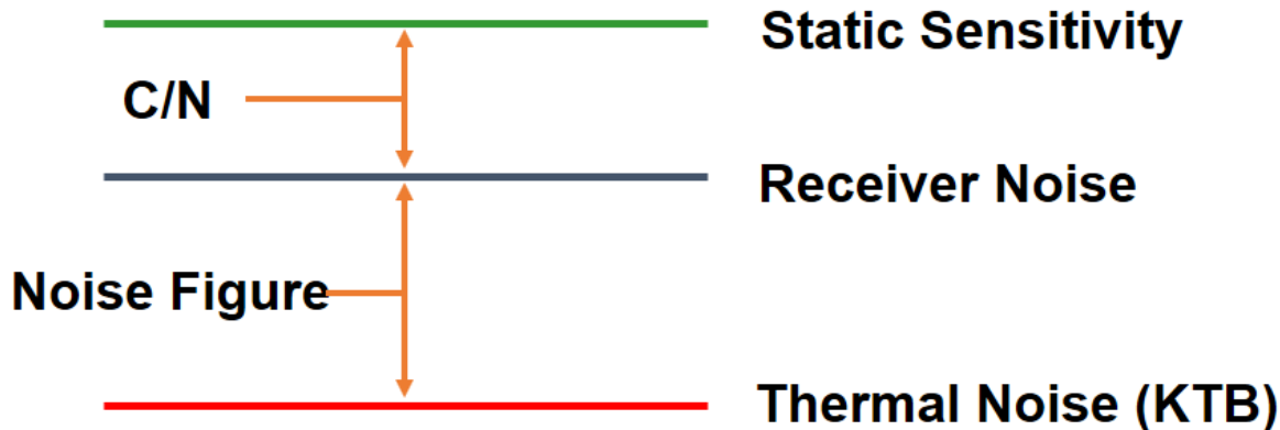
Figure 1: Static Sensitivity components
